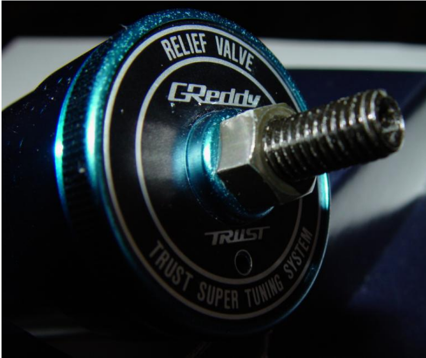
Pic 2: Top View ... see "locking nut" (Size 12M) and "adjusting screw" (Size 4M)
